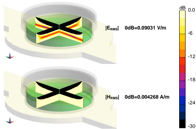
Figure 9: |E_{RMS}| and |H_{RMS}| distribution centered in the petri dish #1. 0 dB are set to the maxima value found on the bottom core (monolayer cells).
